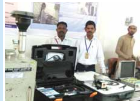
PAPL equipment noise meter and LUX meter used for measuring ambient Noise and Light intensity at workplace
